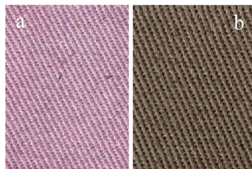
FIGURE 1. Cotton fabrics decorated with (a) Au nanoparticles synthesized using 1% citrate and (b) Pt nanoparticles. Both specimens were produced by electrostatic assembly.
